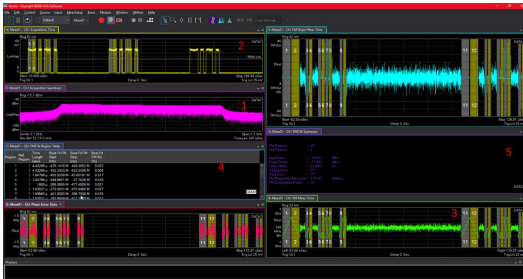
Figure 15. One VSA capture provides information for multiple simultaneous measurements.
