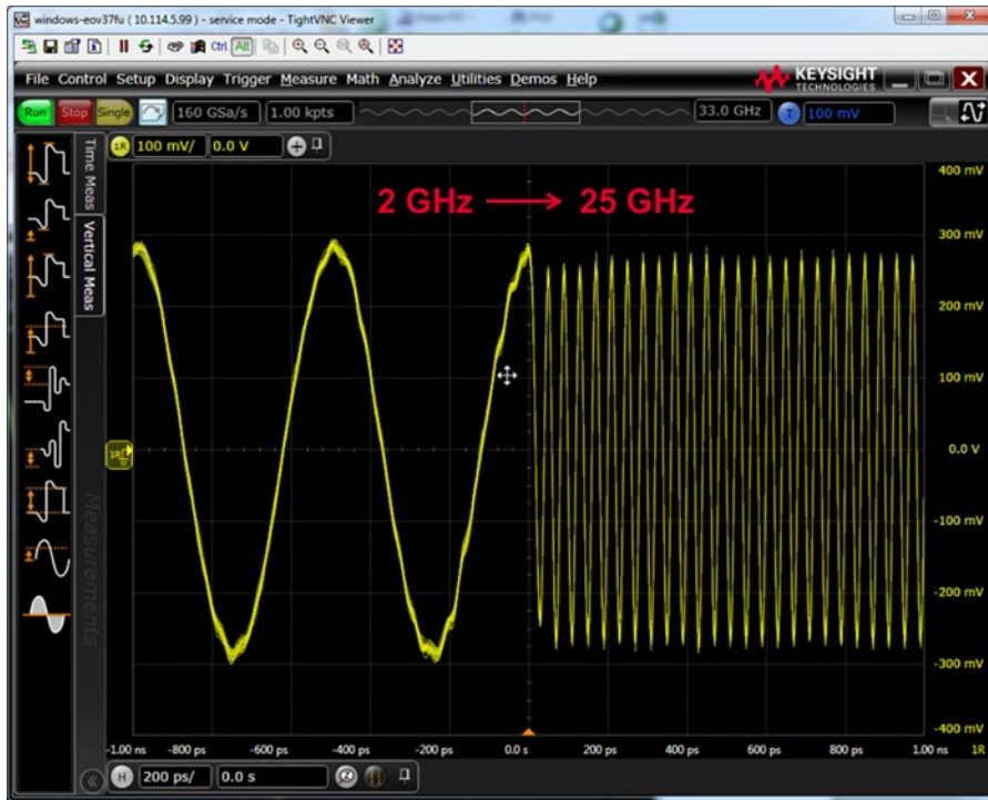
Figure 7. A waveform where frequencies are switched from 2 GHz to 25 GHz with less than 5 Ops
