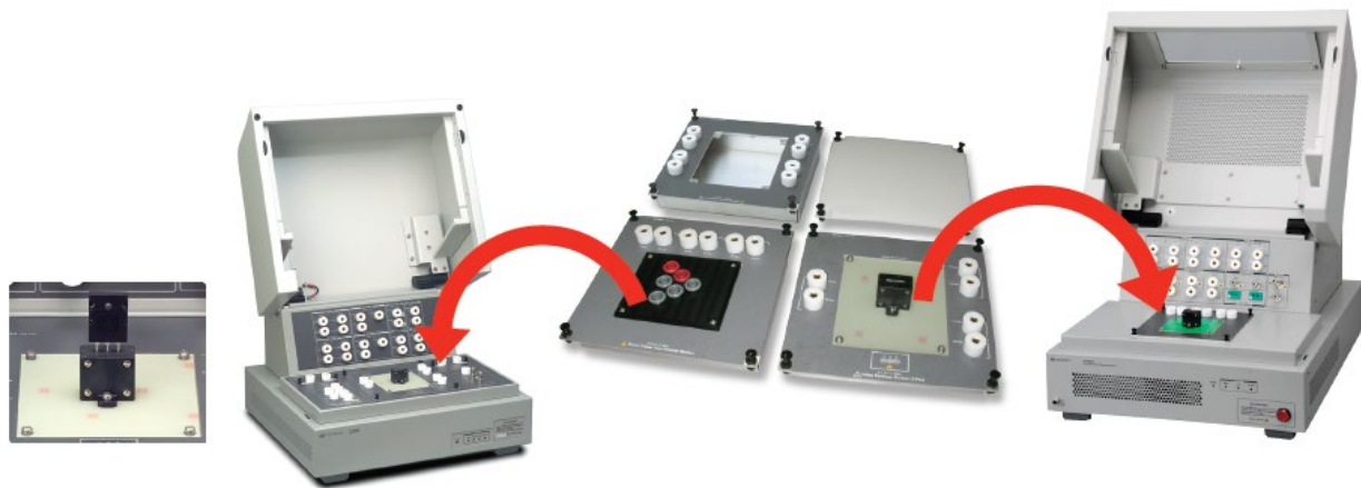
Figure 28. Both test fixtures (N1259A and N1265A) support a variety of different package types
