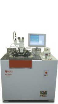
Figure 20. High-power wafer prober control
