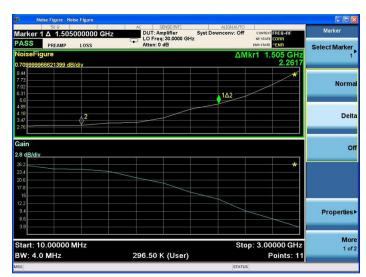
Figure 10. Noise figure measurement
