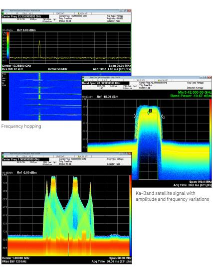
Frequency-hopping LTE-Advanced uplink signal
