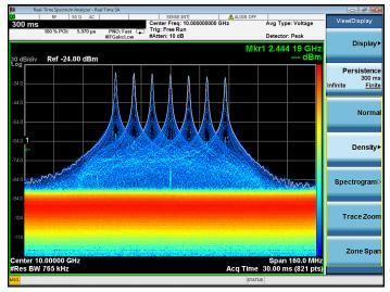
Figure 2. View a fast-hopping radar signal
