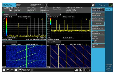
Figure 7. Narrow band frequency domain analysis of a pulse signal changing frequency over time while simultaneously maintaining a wider span for accurate pulse timing measurements
