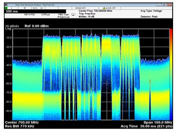
Figure 11. 5-carrier LTE-Advanced signal with in-band and out-of-band interference
