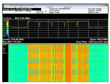
Figure 9. Spectral analysis of an LTE signal where, without demodulation, you can see the signal, control and synch structures are present.
