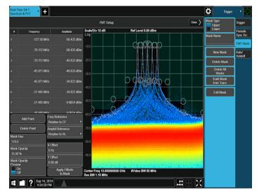
Figure 3. Use FMT to identify signals in frequency hopping pulses. UXA's multitouch user interface significantly simplifies setting up the FMT.
