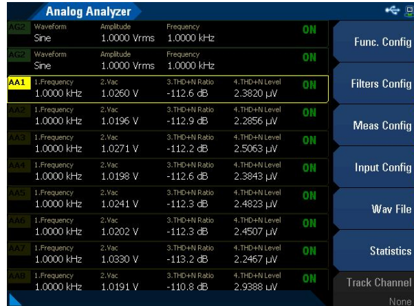
Figure 5. The U8903B's GUI, showing 8 analyzer channel measurements.
