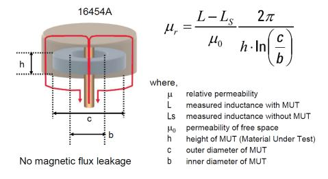
Figure 18. Inductance measurement method
