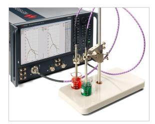
Figure 11. Coaxial probe system
