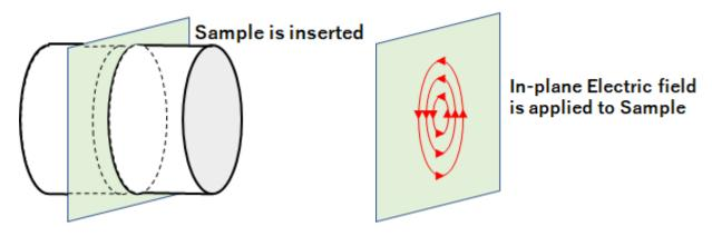
**Schematic diagram of a split cylinder resonator.** The split cylinder resonator is simply two metal cylinders (grey) cut in the middle to allow for a sample (green).
