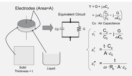
Figure 16. Parallel plate method
