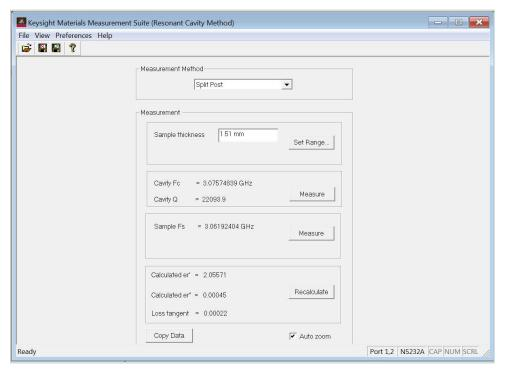
Figure 10. Resonant cavity method user interface
