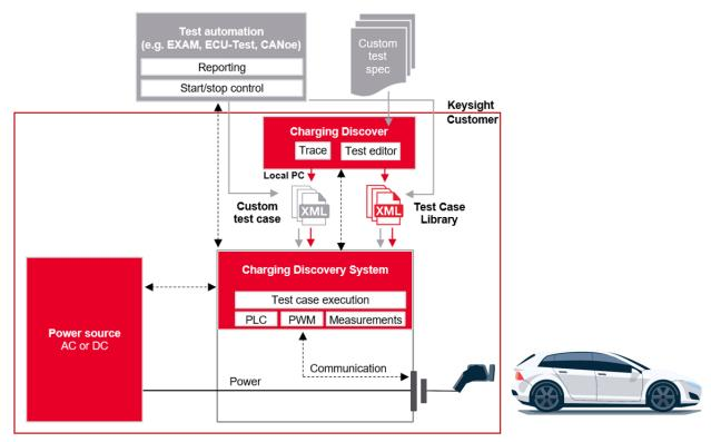
The following figure shows the interface topology of CDS with Expert Mode:
