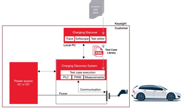
Figure 5. Interface topology of CDS with basic functionality.
