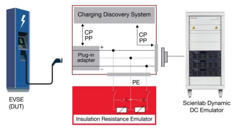
Figure 3. System topology including Scienlab Isolation Resistance Emulator.
